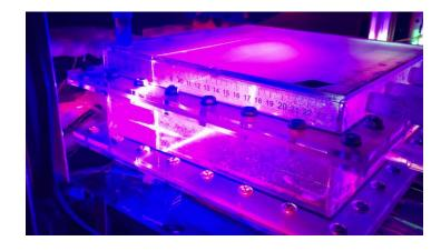
Only the vertical vorticity of lower layers were measured Scanning period: 12 seconds
