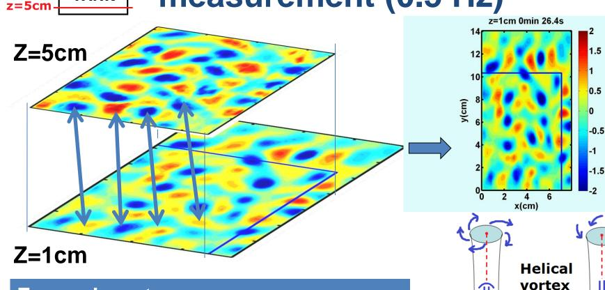
For each vortex, vorticity are vertically antisymmetric, with comparable strength
